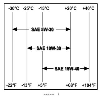
**NOTE:** In areas where prolonged periods of extreme temperatures are encountered, local lubricant practices are acceptable; such as the use of SAE 5W-30 in extreme low temperatures or SAE 50 in extreme high temperatures.
