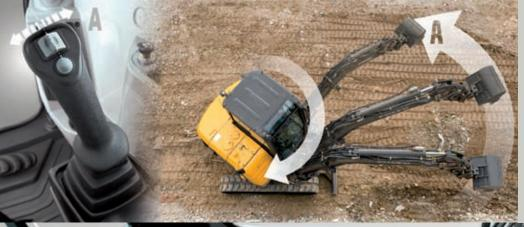
Easy grip joysticks with proportional control. Slew and offset are efficiently combined.
