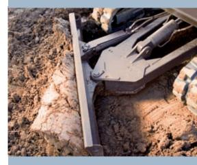
Hydraulic angle blade rotates to save time.
